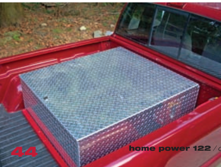
In the bed—a custom battery box holds eighteen T-145s.
