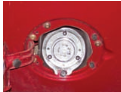
The original gasoline filler cap was replaced by a 240 VAC plug.
